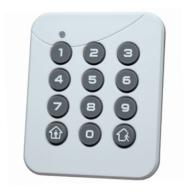
This battery powered Clare Wireless Pinpad is simple-to-install and allows for local control of the security panel. Pinpads can be installed in nearly any location for complete control over arm stay, arm away, panic modes, and more.
