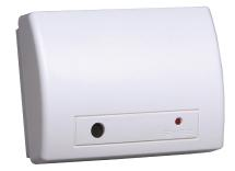
The Glass Break Detector identifies the sound of breaking glass. It can be mounted anywhere in the home that is from 4-25 ft from doors & windows to cover an entire room. Powered by a single 1550 mAH battery, the detector operates for up to 4-6 years. The glass break detector is ideal for extending coverage over a large area in a home or business.
