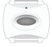
**Enroll** the panic by placing the panel into wireless enrollment mode and pressing the red panic button. Alternatively, the panic can be enrolled by scanning its bar code using the Install Assist App or by entering its 8-character serial number on the interactive service provider's web portal.
