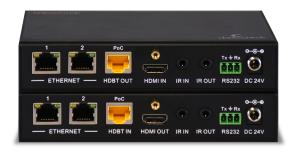
The extender set uses HDBaseT technology to transmit HDMI signals from a single source (i.e., a cable or satellite set top box, Blu-ray player, game console) over conventional CAT 5e/6/7 UTP over distances up to 100 meters (328 ft)\*. Each PoCcapable set is HDCP 2.2 compliant, supports 4K x 2K, 1080p, and 3D and provides bi-directional IR and RS232 control and Ethernet to the room.
