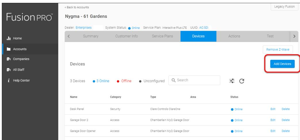
4. Select the device category (**Access**) and then the device type (**Z-Wave Device – Access**).
