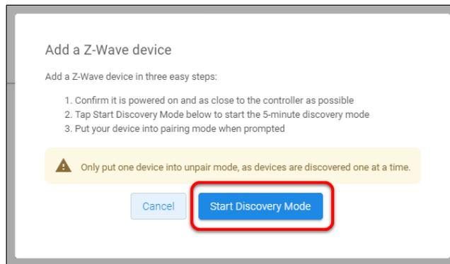
A popup displays waiting for a notification from the device, pair the Z-Wave device according to the manufacturer's instructions for each device.
