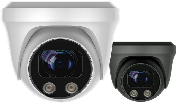
Featuring a 4MP, Sony® Starvis™ image sensor, this Performance Series ClareVision Turret camera includes a 2.8 mm lens with a maximum recording resolution of 2560 x 1440p at a stable 30 FPS. The camera includes support for True WDR and includes a 32 GB micro SD card for local, onboard storage.
