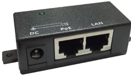
A Power-over-Ethernet (PoE) injector eliminates the need to run dedicated power wires to ClareVision Plus PoE cameras by introducing DC voltage onto the CAT cable that carries the video stream. Fully compliant with the IEEE 802.3af (PoE) standard, this unit eases and speeds the installation of 802.3af and surveillance cameras. Includes LED indicator for power status.
