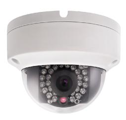
The CV-B13D10-ODI is an affordable mini-dome ideal for outdoor deployment in mainstream video surveillance applications. Powered via PoE or 12V supply, the compact (4.4" dia x 3.2") ONVIF-compliant camera provides up to 1.3 megapixel (1280 x 960) resolution, onboard IR illumination to 30 meters, digital WDR, and an IP66 sealed, vandal-proof housing.
