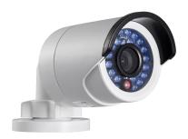
The 2 MP IP bullet camera is a 4 mm fixed-lens camera with IR LED, range up to 30 meters. Features include PoE, a 4 mm fixed lens, and IP67 sealed housing. The small form factor allows for covert installs where tampering is of low concern.
