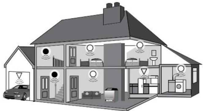
Figure 2: Detector placement single level
