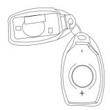
3. Use a fingernail/fingertip to push the battery out of the casing, noting the polarity of the battery.
