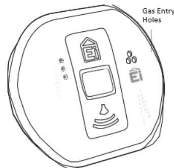
Within seconds, the red LED begins to flash (as per Table 2) confirming that the alarm has detected the CO.
