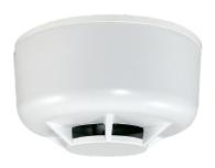
Rate of temperature rise is often an indicator of fire, even before smoke reaches the smoke alarm. The ClareOne Rate of Rise Heat Detector uses Thermistor-based sensing to detect and report rapid rising heat conditions or when temperature reaches 135°F. The detector can be mounted almost anywhere to detect a rise in heat conditions.
