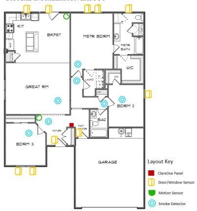
Note: The maximum distance over which a sensor and the panel can communicate may be reduced when the equipment is installed in a typical home. Placement of the sensor, building materials and construction, location of mirrors and other RF interfering/blocking devices can all reduce the overall range.
