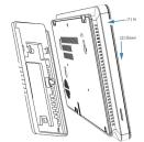
Press the panel onto the mounting bracket, and then slide the panel downward.
