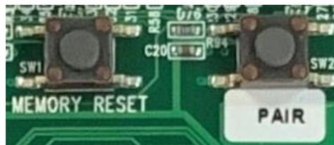
**Memory Reset Button:** The Memory Reset button clears the HWIM's memory and returns it to the factory default settings. The Memory Reset button is also used to enable/disable the communication timer delay for Zones 1 and 2.
