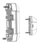
Mount the magnet into the desired location making sure the magnet alignment mark lines up with the sensor mark.
