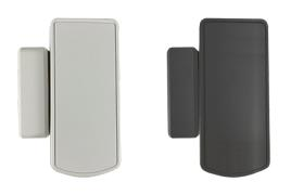
The ClareOne Mini Door/Window Sensor places intrusion alerts in all common entry points. This magnetic sensor's small form factor is designed to fit seamlessly alongside a door or window frame. When the door or window is opened, the magnetic contact is disrupted, and the sensor transmits an alarm notification to the ClareOne panel.
