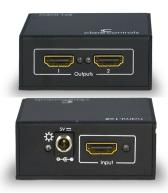
The Clare HDMI 1x2 splitter is a high-performance distribution amplifier, designed to allow users to direct high definition video from a single source to two HDTVs, monitors, projectors, etc.
