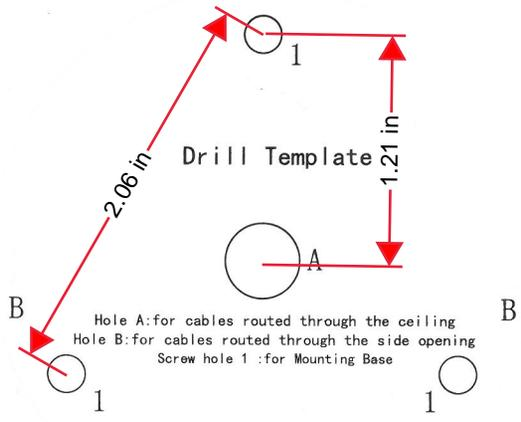
Hole A: for cables routed through the ceiling
