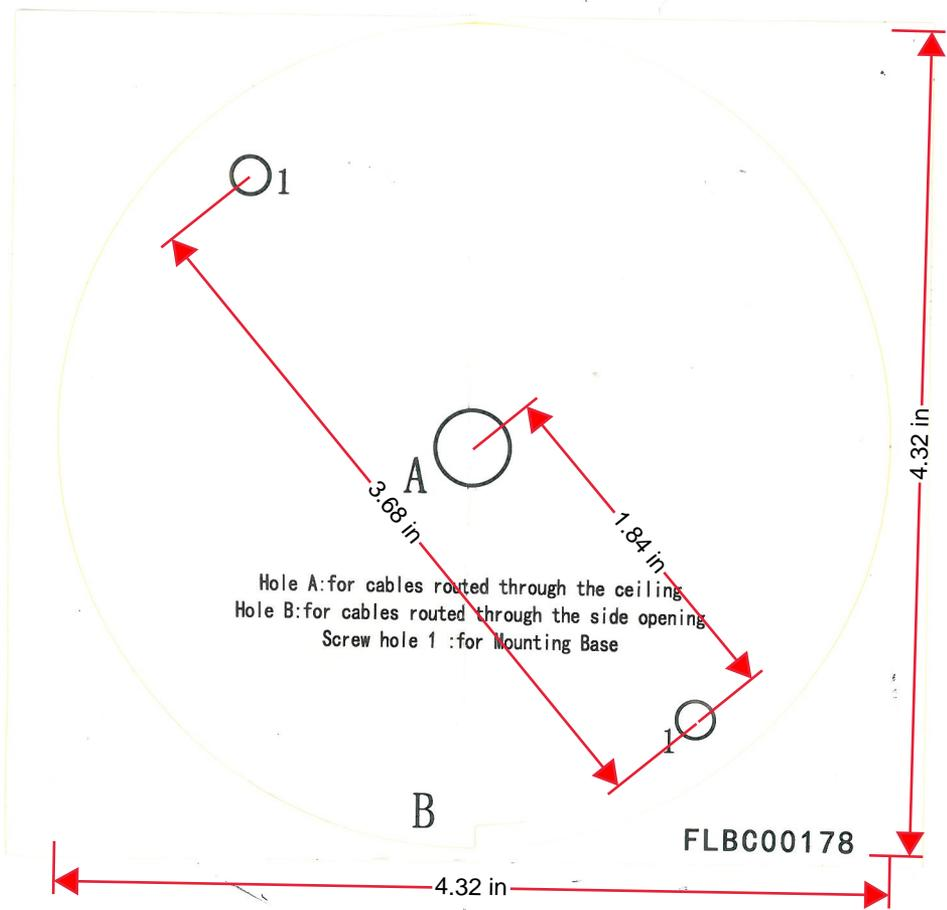
Hole A: for cables routed through the ceiling
