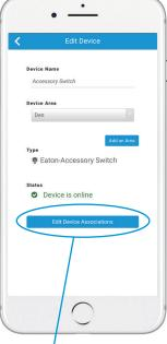
Next, tap on the accessory switch or dimmer you wish to associate. (The accessory device will control the master device.)
