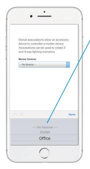
You can pair and configure ClareVue lighting keypads using Install Assist. Simply pair the keypad the same way you'd pair any other lighting device, name each button, and configure it's function.
