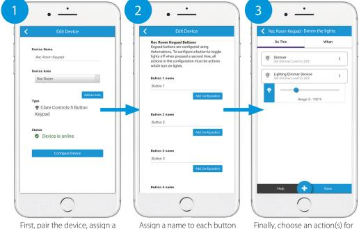
First, pair the device, assign a name, and add it to an area. Tap Configure Device.
