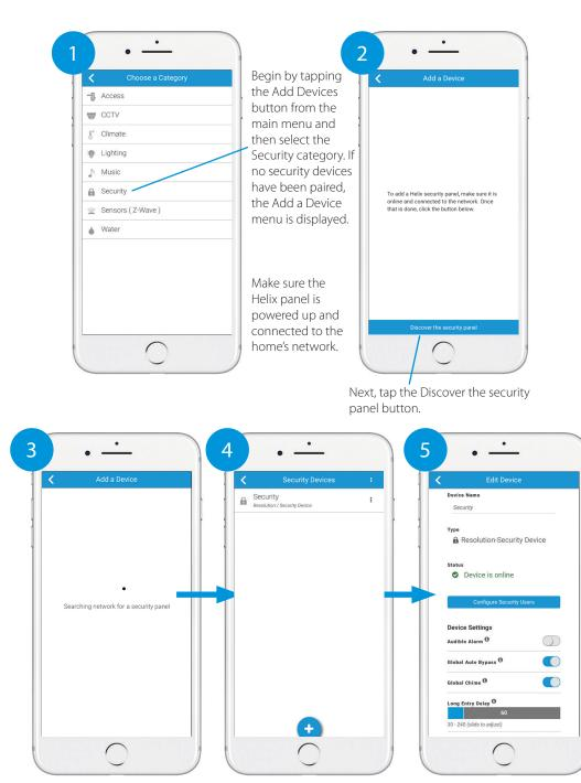
Install Assist searches for a connected Helix security panel.
