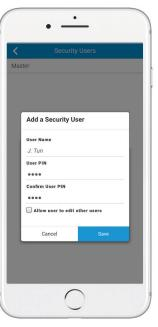
To edit the master user code, simply enter a new pin code and verify. Tap Save to finish. Creating a new user is just as simple. Enter a user name, and assign a PIN code. After confirming the PIN code, tap Save to finish. Using Install Assist, installers or homeowners can quickly access devices in a certain location by adding an area. Areas can be added quickly in just a few steps.
